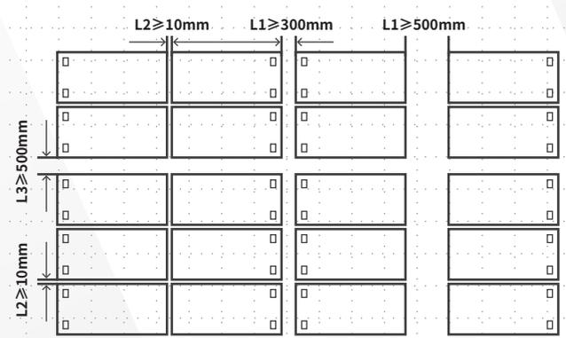
1. Spacing with the junction box terminal on the top: 300mm.
