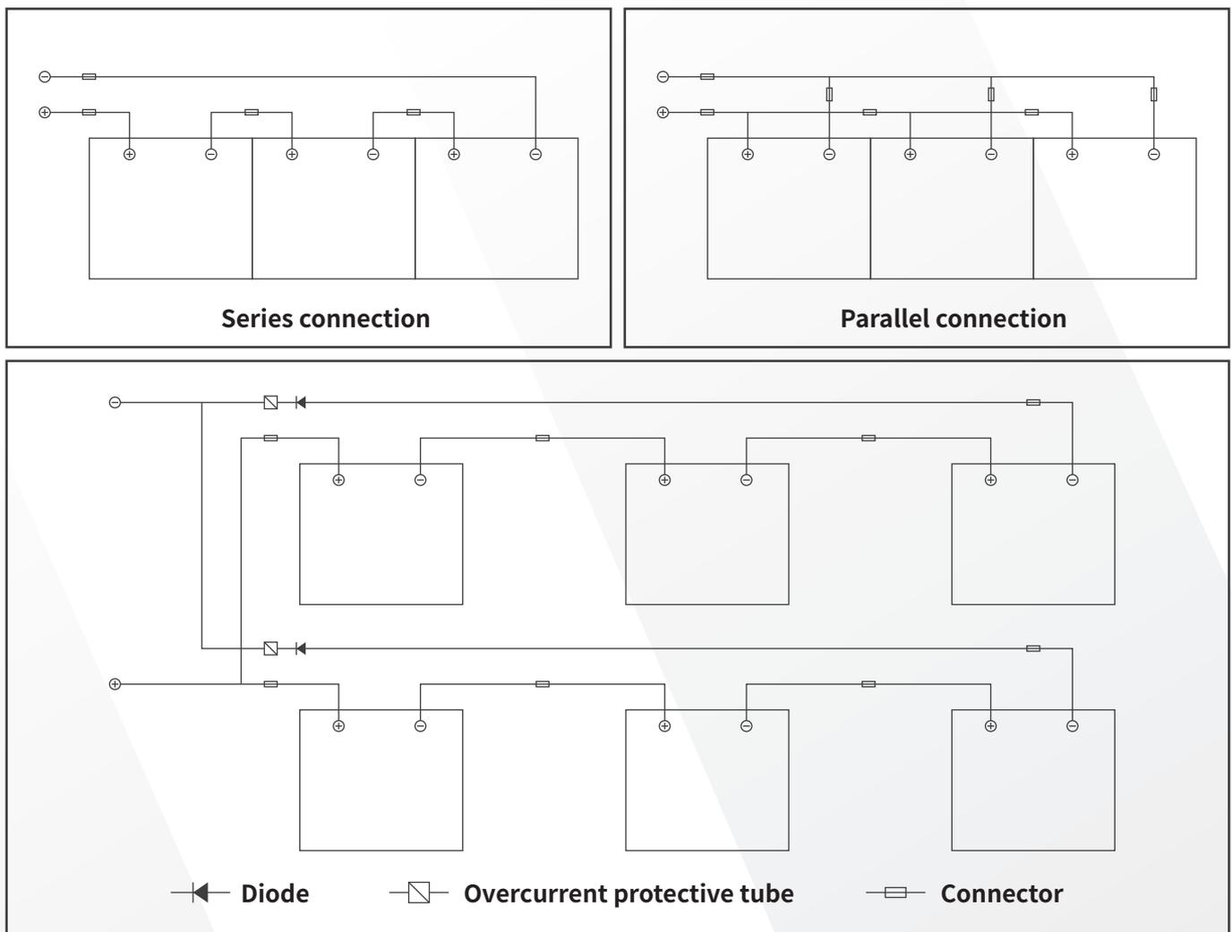
**Circuit Diagram of Series Connection and Parallel Connection**
