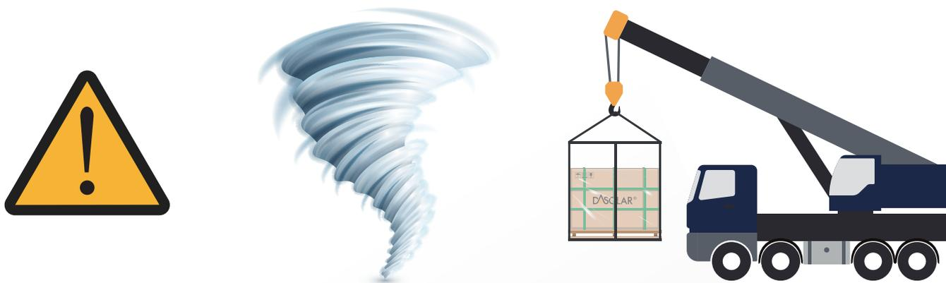
Please do not hoist the Module in any adverse weather conditions, such as strong wind greater than scale 6 (Beaufort scale), heavy snow or heavy rain. At most 2 trays of modules can be hoisted together if they are in horizontal packing.
