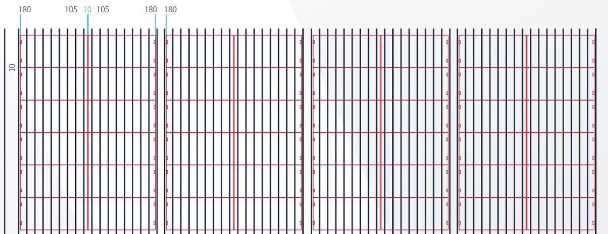
**YX-25-210-840 trapezoidal color steel tile - layout schematic**
