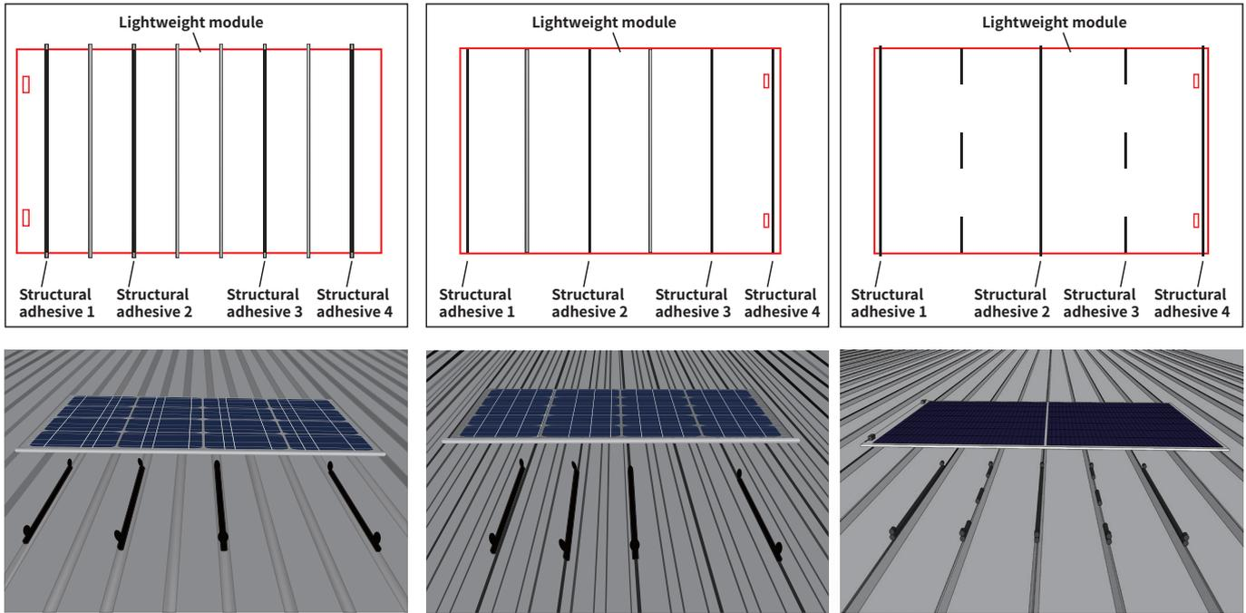
**Trapezoidal color steel tile installation schematic**
