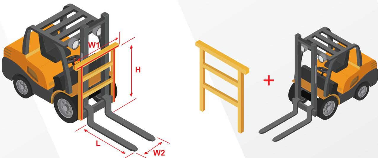
The fork length (L) shall be N1.0m, and fork interval (W2) shall be adjusted to approach the two corners of the tray to the greatest extent.
