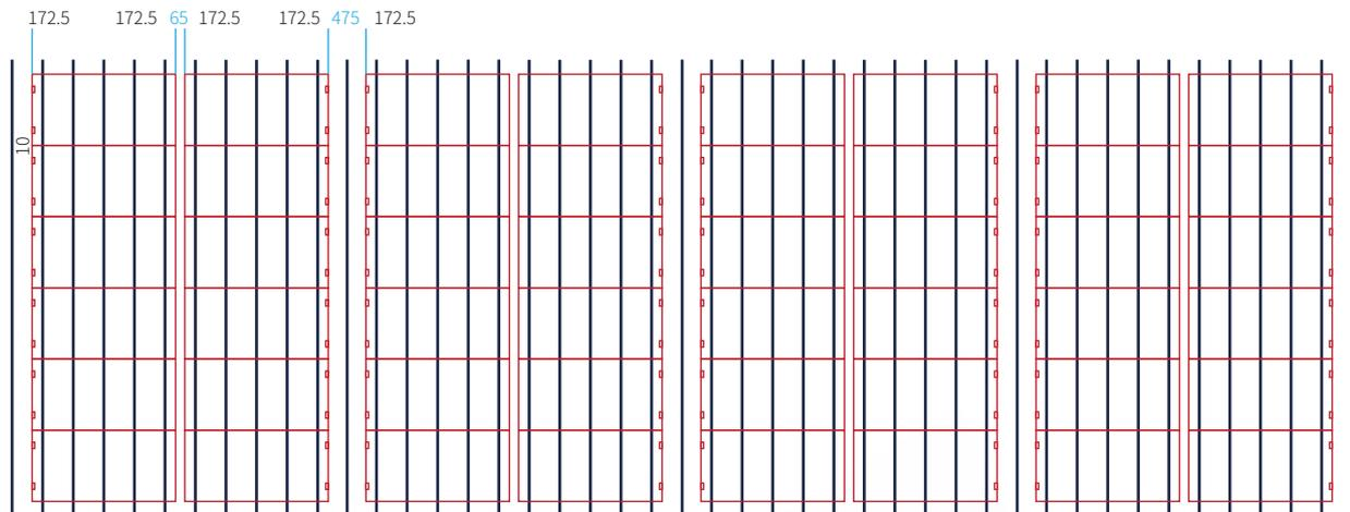
**YX51-410-820 angle color steel tile - layout schematic**
